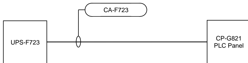
Figure 7-3: Instrument Cable Identification Example – Identified Equipment
